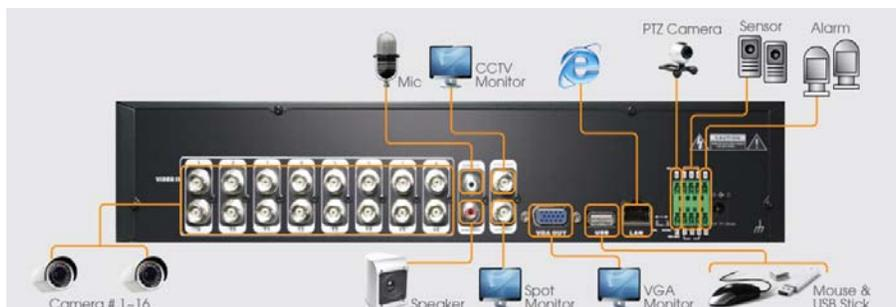
**Warning !** ※ Depending on the grounding, the BNC cable connecting to the camera has danger of electric shock. Shut down the system power completely and unplug the power cable before connecting BNC cable to BNC port of the system.
